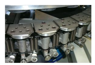
This system allows to lift the cans in a perfectly vertical way as far as they reach the rubber heads and to keep them in position during the entire duration of the test. In this way the cans are positioned without the necessity of a containment tool under the rotating table and so this feature allows a quick can size change
